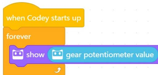
Method 2: Connect your device to Codey, tick the box before **the gear potentiometer value** block under Sensing category.
