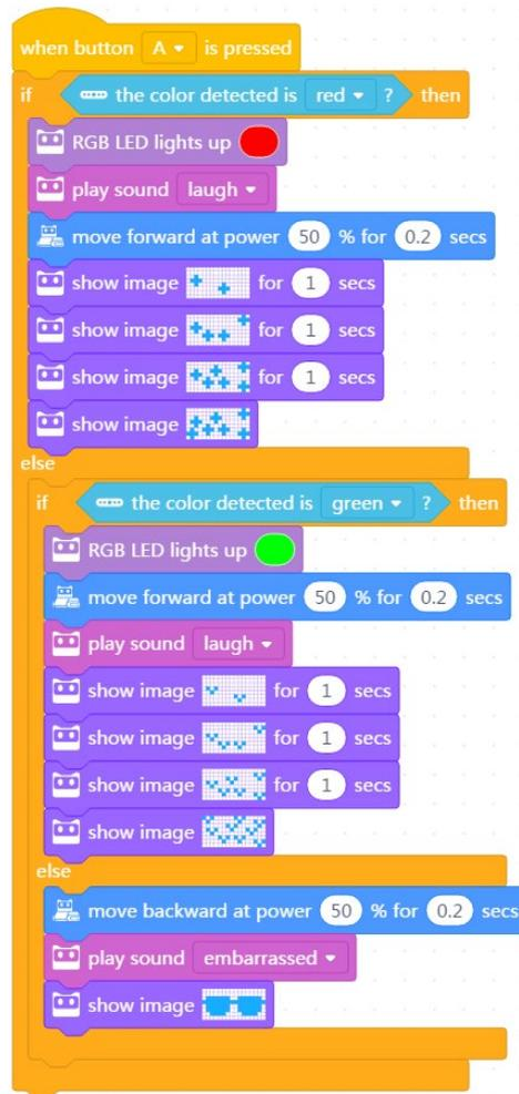
Explain how to program the color sensor: "If we want to program the color sensor, we'll need to use these blue Sensing blocks. We can pull the drop-down menu to reset the color to be detected."
