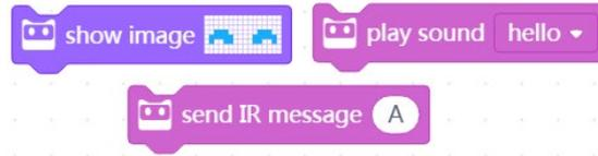
2. Device-Codey2: When it starts up and receives the IR message "Hi", Codey2 waits for 1 second, makes a response (like a smiley face and/or a laughing sound), and then sends an IR message "Hello".
