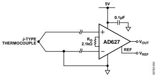
Figure 51. Amplifying Bipolar Signals with Low Common-Mode Voltage
