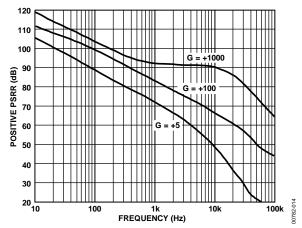
Figure 16. Positive PSRR vs. Frequency ( $V_S = 5 V, 0 V$ )
