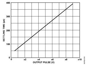
Figure 20. Settling Time to 0.01% vs. Output Swing, G = +5,  $R_L = 20 \, k\Omega$ ,  $C_L = 100 \, pF$
