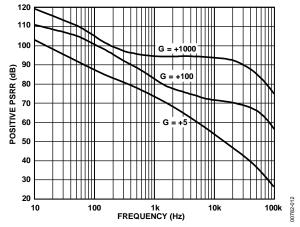
Figure 14. Positive PSRR vs. Frequency, ±5 V
