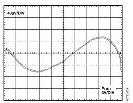
Figure 31. Gain Nonlinearity, Negative Input,  $V_S = \pm 15 \text{ V}, G = +5 \text{ (1.5 ppm/DIV)}$
