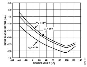
Figure 8. Input Bias Current vs. Temperature
