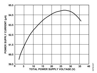
Figure 9. Supply Current vs. Supply Voltage
