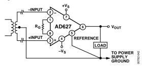
Figure 44. Ground Returns for Bias Currents with Transformer Coupled Inputs
