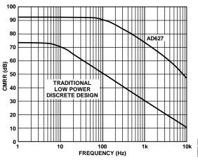
Figure 2. CMRR vs. Frequency,  $\pm 5$  Vs, Gain = +5
