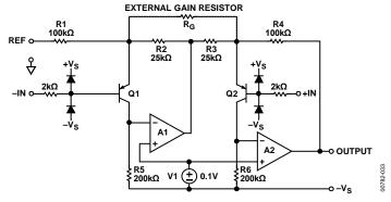
Figure 35. Simplified Schematic
