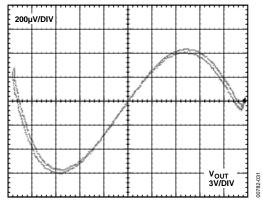
Figure 33. Gain Nonlinearity, Negative Input,  $V_S = \pm 15 \text{ V}, G = +5 (7 \text{ ppm/DIV})$
