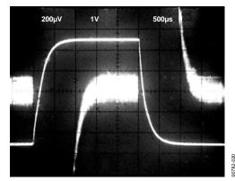
Figure 22. Large Signal Pulse Response and Settling Time, G=-1000,  $R_L=20~k\Omega, C_L=100~pF~(10~\mu V=0.01\%)$
