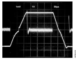
Figure 18. Large Signal Pulse Response and Settling Time, G = –5,  $R_L$  = 20 k $\Omega$ ,  $C_L$  = 100 pF (1.5 mV = 0.01%)
