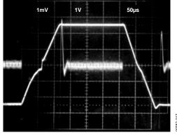
Figure 19. Large Signal Pulse Response and Settling Time, G=-10,  $R_L=20~k\Omega$ ,  $C_L=100~pF$  (1.0 mV = 0.01%)
