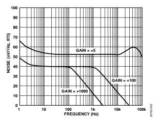
Figure 5. Voltage Noise Spectral Density vs. Frequency
