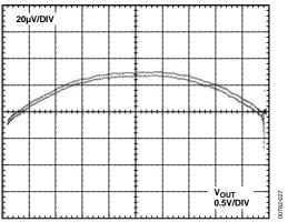
Figure 29. Gain Nonlinearity, Negative Input,  $V_S = \pm 2.5 \text{ V}, G = +5 \text{ (4 ppm/DIV)}$
