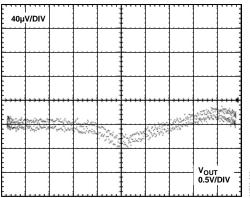
Figure 30. Gain Nonlinearity, Negative Input,  $V_S = \pm 2.5 \text{ V}, G = +100 \text{ (8 ppm/DIV)}$
