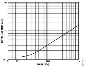
Figure 17. Settling Time to 0.01% vs. Gain for a 5 V Step at Output,  $R_L=20~k\Omega$ ,  $C_L=100~pF$ ,  $V_S=\pm5~V$
