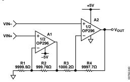
Figure 42. 0.1% Resistor Mismatch Example
