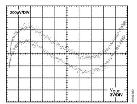
Figure 34. Gain Nonlinearity, Negative Input,  $V_S = \pm 15 \text{ V}, G = +100 \text{ (7 ppm/DIV)}$
